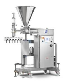
The electronic-volumetric depositor mod. DVE has a pumping system with a syringe.
